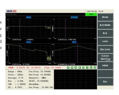
■ Long-distance detectivity 6419 can detect the optical fiber line nearly 80km.
